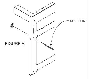
2) Using drift pins on top and bottom align bolt holes. (FIGURE B)
