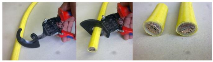
Remove of the insulation: With a good knife, the braid have to be cut together with the silicone insulation and can be removed properly:
