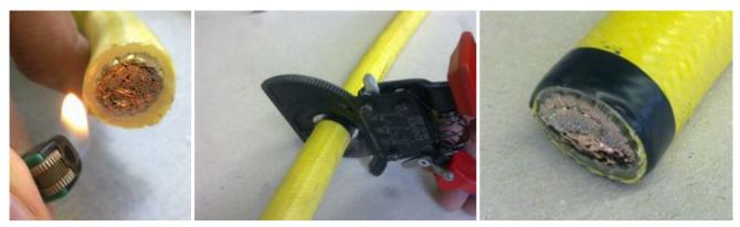
Finally, it's also possible to purchase Siwo-Kul-Sil where the braid is gluing on the silicone insulation.
