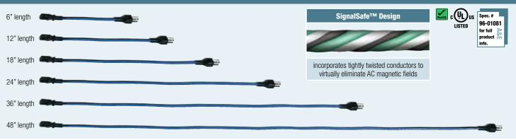
Unwanted AC magnetic fields can infiltrate the signal path & cause problems in your installed systems. Power cords under load, especially long ones, are sources of AC magnetic fields. To minimize these effects in your systems, look for the stripe that identifies the SignalSafe technology. SignalSafe power cords feature tightly twisted conductors to reduce the effects of AC magnetic fields.
