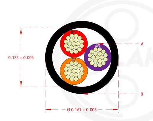
A: 18 AWG 3 Conductors Plenum Rated SGPVC Insulated
