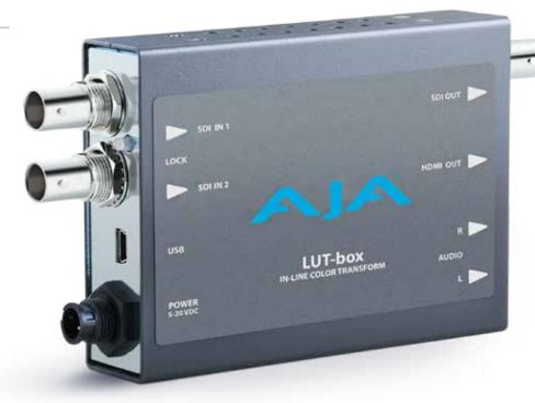
LUT-box supports 3D color correction for accurate monitoring of video signals. Users can load 17x17x17 3D LUTs via USB using the free MiniConfig software on either Mac or Windows. Simultaneous outputs allow you to utilize both HDMI and SDI monitors from a single LUT-box. Embedded audio is passed through to the outputs and a 2-channel RCA analog output allows easy audio monitoring of embedded audio.
