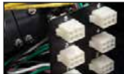
Quick Disconnect Electrical Breakout
