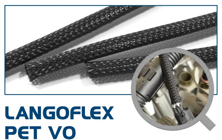
LANGOFLEX PET V0 is a tough, lightweight expandable sleeving made of PET .010" (0.25mm) monofilaments braided into a cylindrical sleeve.
