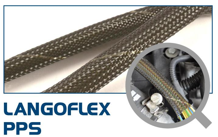
LANGOFLEX PPS is a high temperature, nonflammable and lightweight expandable sleeving made from 0.25mm diameter of polyphenylene sulfide (PPS) monofilament.
