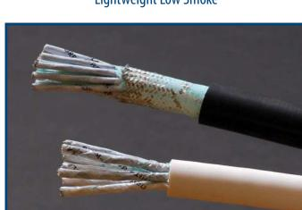
"0" in the part number indicates that the cable has an optimized shield. The optimized shield is a single braid that is constructed to provide the same shielding performance as a double braid in the MIL-DTL-24643 specification, while saving weight and reducing the cable diameter. The optimized
