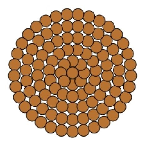
**Description:** Ropelay Stranded Conductor 16 AWG 105/36 TC
