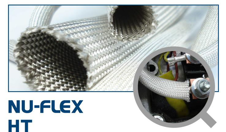
Delfingen NU-FLEX HT is a tightly woven, flexible, continuous filament electrical grade 100% fiberglass braid heat treated to remove all organic contaminants and to set the glass braid for end-fray resistance.
