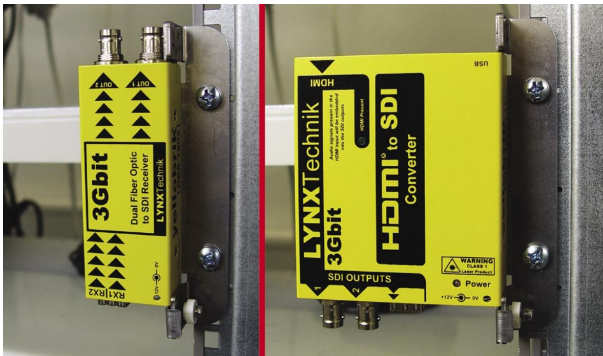
Bracket shown mounted on 19" rack rails
