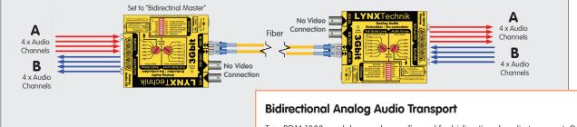
Two PDM 1383 modules can be configured for bidirectional audio transport. One module is switched to be a "Bidirectional Master"
