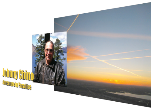
Two key layers and a background source can be simultaneously combined to produce the program output
