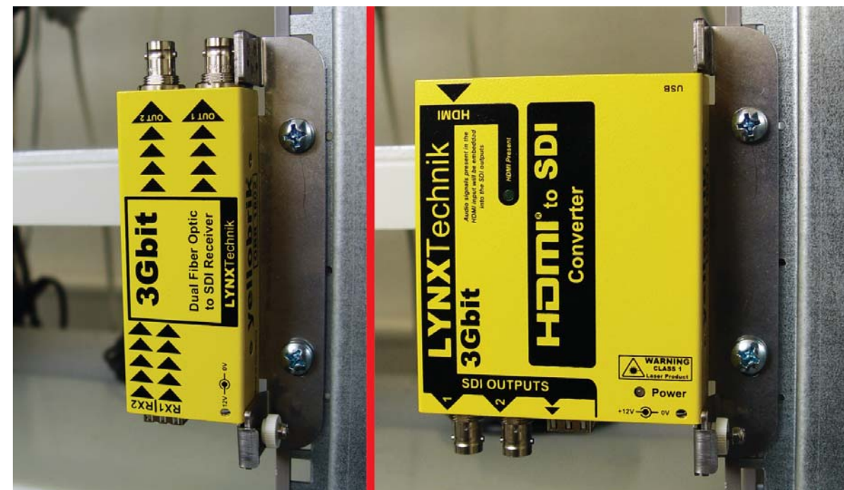
Bracket shown mounted on 19" rack rails
