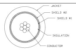
DBRF240SF Super-Flexible Low Loss 50 Ohm Coaxial Cable that is used for Jumper assemblies in Wireless Communications Systems, Antenna Feeder Runs and any application requiring a Low Loss RF Cable
