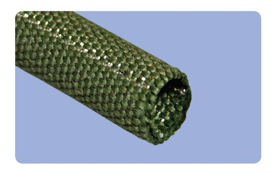
**ROUNDIT® 2000 NX** is a woven combination of Nomex® and PPS (polyphenylene sulfide). The Nomex®/PPS blend in a flat weave construction gives ROUNDIT 2000 NX a rugged yet smooth texture and appearance for high temperature bundling and abrasion resistance. This product is rated to +200°C (+392°F) and is non-halogenated.
