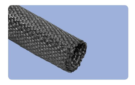
**ROUNDIT® 2000** is a woven blend of polyester monofilaments and multifilaments. The monofilament/multiflament blend in a flat weave construction gives ROUNDIT 2000 a rugged yet smooth texture and appearance. This product is rated to +125°C. Roundit has many applications in the aeronautical, marine, electronic, furniture accessory and general manufacturing industries.
