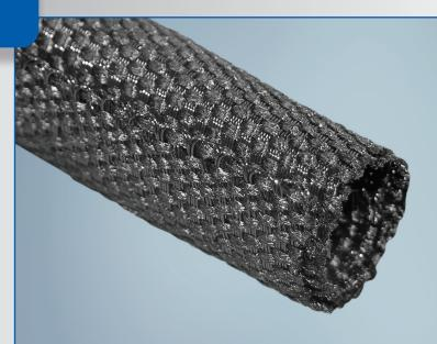
**ROUNDIT® 2000** is a woven blend of polyester monofilaments and multifilaments. The monofilament/multiflament blend in a flat weave construction gives ROUNDIT 2000 a rugged yet smooth texture and appearance. This product is rated to +125°C. ROUNDIT has many applications in the aeronautical, marine, electronic, furniture accessory and general manufacturing industries.
