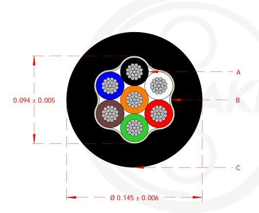
A: 26 AWG 7 Conductors 19 Strands Tinned Copper Wire with FEP Insulation
