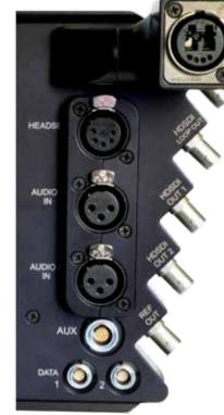
At the rear of the unit are XLR's for Audio MIC inputs 1 and 2 and a 5-pin XLR for Intercom.
