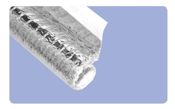
**Therm-L-Wrap**<sup>™</sup> is a self-wrapping, reflective sleeve designed to provide thermal protection from both radiant and convective heat. Composed of a woven fiberglass base fabric and a lamination of aluminum foil, the product can withstand convective heat soaks up to 200°C and simultaneously protect critical components from radiant or reflected heat.
