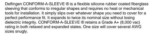
CONFORM-A-SLEEVE ® can be used over rectangular wire in form wound coils, over bus bars, bus bar connections and motor lead connectors. It is an excellent choice for high reliability protection in wire harnesses and can be used as an insulator over brazed or soldered splices and hard to insulate irregular shapes. Additionally, CONFORM-A-SLEEVE ® provides a superior alternative to heat shrinkable tubing, acrylic tubing and many types of tape applications.
