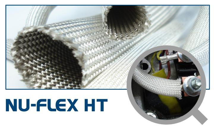
Delfingen NU-FLEX HT is a tightly woven, flexible, continuous filament electrical grade 100% fiberglass braid heat treated to remove all organic contaminants and to set the glass braid for end-fray resistance.
