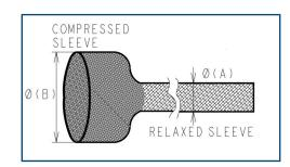
Diameter is measured over a mandrel. Length for cut pieces is measured in a relaxed position.
