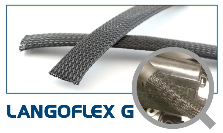
LANGOFLEX G is a tough, lightweight expandable sleeving made of PET .010" (0.25mm) monofilaments braided into a cylindrical sleeve.
