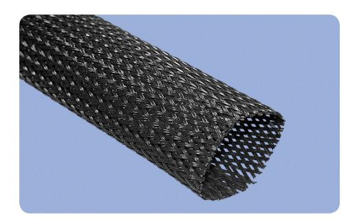
**Expando® PT & Expando® PT Plus** are tough, lightweight oversleeves used to protect cable assemblies, hoses and wire harnesses from chafing, cutting and abrading. The open-braid construction of Expando products enables each size to expand to fit several application shapes and diameters. This open-textile construction also makes them highly flexible and resistant to trapping water, heat and humidity.
