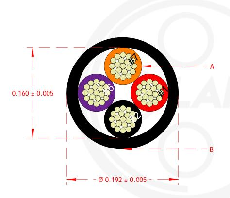
A: 18 AWG 4 Conductors 19 Strands Bare Copper
