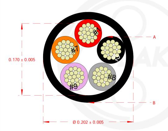
A: 18 AWG 5 Conductors 19 Strands Bare Copper
