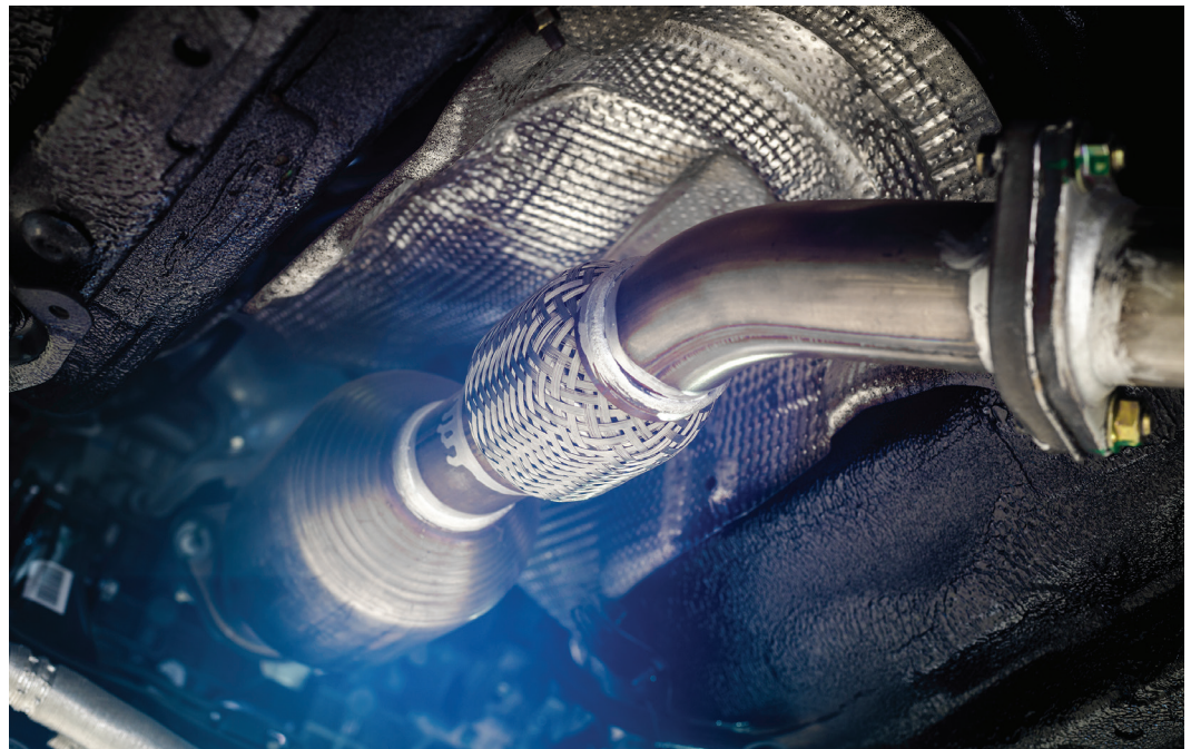
Stainless Steel sleeving is used in applications such as expansion joints, where constant movement and high temperatures require a flexible, indestructible covering.
