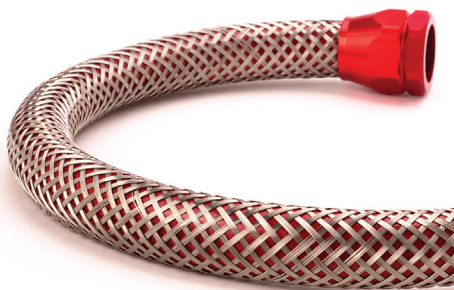
Stainless Steel sleeving is used in applications such as expansion joints, where constant movement and high temperatures require a flexible, indestructible covering.
