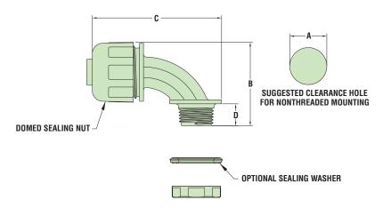
Material<br/>CertificationsNylon 6/6<br/>Listed under Underwriters' Laboratories File E28430Image: Standard Standards Association<br/>File 84579 and 81067Flammability Rating<br/>Temperature Range94V-2<br/>-22°F (-30°C) to 221°F (105°C)IP RatingIP 68 up to 70 psi (5 bar) water pressure
