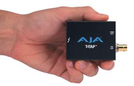
Small and simple to use, T-TAP connects direct to your computer system via the blazing-fast Thunderbolt connection which provides the bandwidth necessary for full broadcast-quality video and audio output.
