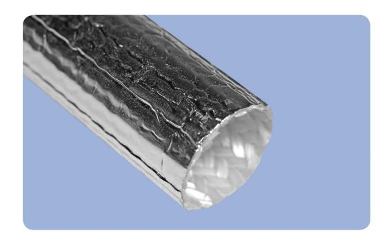
**Therm-L-Lite® FG** is a one-piece fiberglass sleeve that is laminated to an aluminum foil. A special manufacturing process permits the sleeve to boast a virtually seamless and non fraying construction. This features make Thermal-L-Lite FG a low profile solution easily applied to the application it protects. The outer aluminum finish is highly reflective while the inner layer of the fiberglass greatly increases insulating efficiency.
