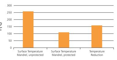
**Heat Source Temperature:** 540°C, 15 mm below ceramic mandrel.
