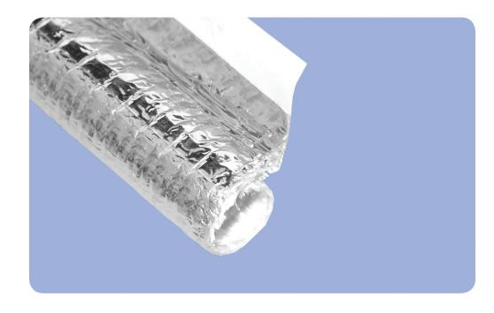
Therm-L-Wrap™66 is a self-wrapping, reflective sleeve designed to provide thermal protection from both radiant and convective heat. Composed of a woven fiberglass base fabric and a lamination of aluminum foil, the product can withstand convective heat soaks up to +200°C (+392°F) and simultaneously protect critical components from radiant or reflected heat.
