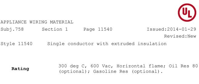
Conductor 30 AWG - 8 AWG, solid or stranded. Nickel plated Copper.
