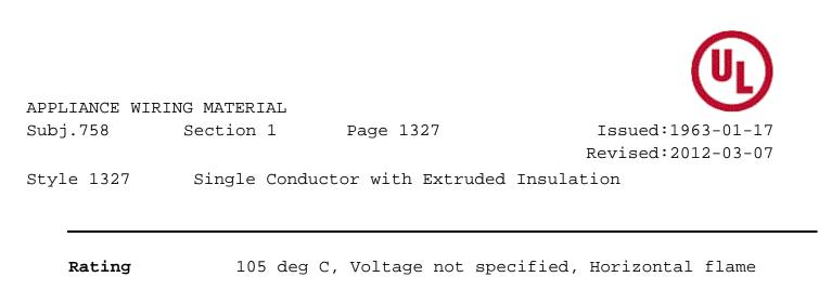
Conductor 30 AWG - 16 AWG solid or stranded
