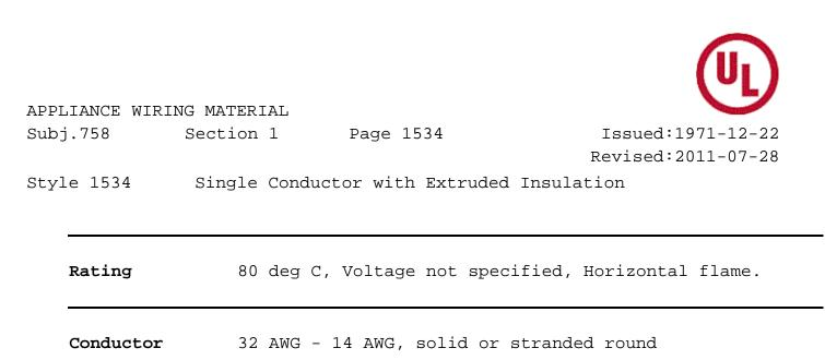
Insulation Extruded XLPVC, 10 mils minimum average thickness, 9 mils minimum thickness at any point
