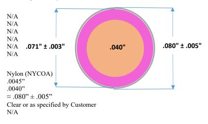
90°C Dry locations 60°C where exposed to moisture or oil. 600 VAC rated 105°C when used as AWM 1316 or 90°C 1000 VAC when used as AWM 1452
