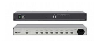
The VM-8H is a distribution amplifier for HDMI signals. It reclocks and equalizes the signal and distributes it to 8 identical outputs.
